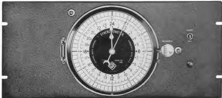
Figure 1. Panel view of the Synchronometer. The Microdial is at the right of the clock face.
